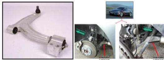
Figure 1: Front Lower Control Arm (FLCA) [6]
