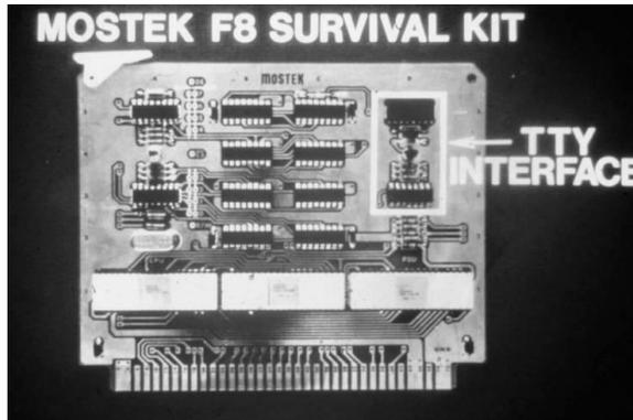
**Figure 3a:** Typical single-board 'evaluation kit'
