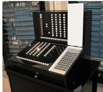
Figure 10: Left: The punch tape reader. Right: The hidden safe implemented in the input-device. With 60 buttons it is possible to control all the components of the new separately. It did not exist in the original Z3.
