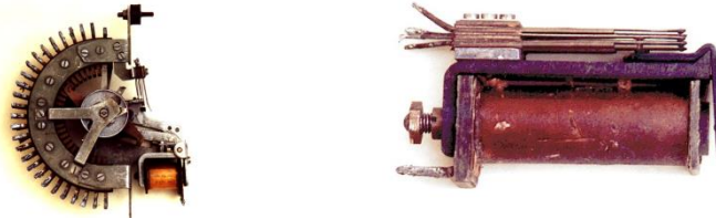
Figure 4: Left: Stepwise relay for the control in order to make, among others, the multiplication by repeated addition. Right: A relay of the Z3.
