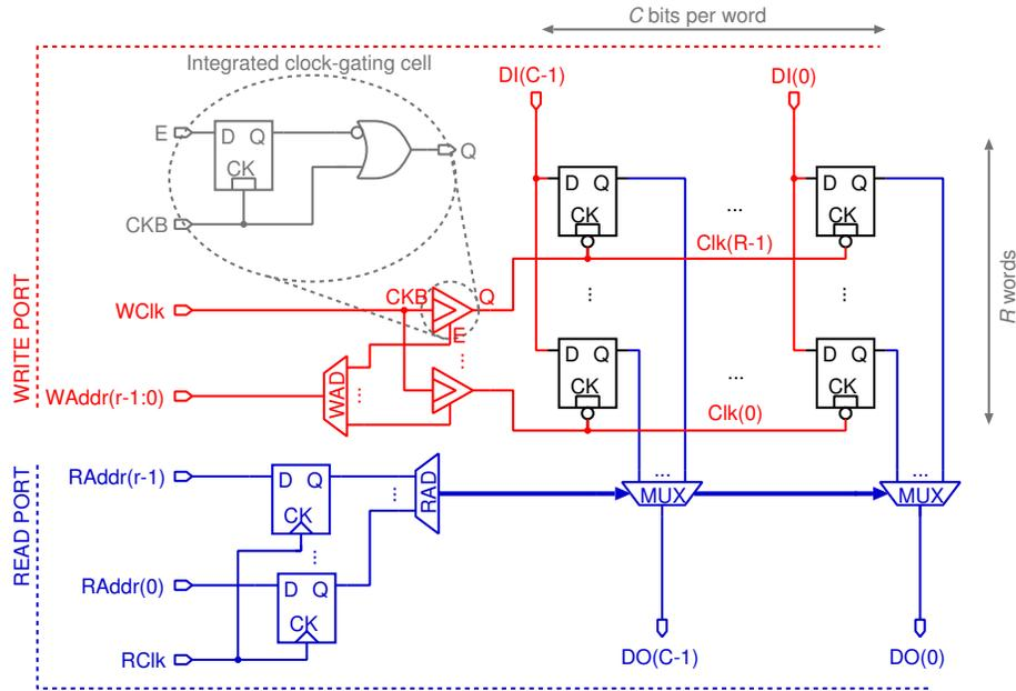
**Fig. 2.** Schematic of the latch array with clock-gates for the generation of write select signals and static CMOS readout multiplexers. The write port is highlighted in red, while the read port is highlighted in blue.
