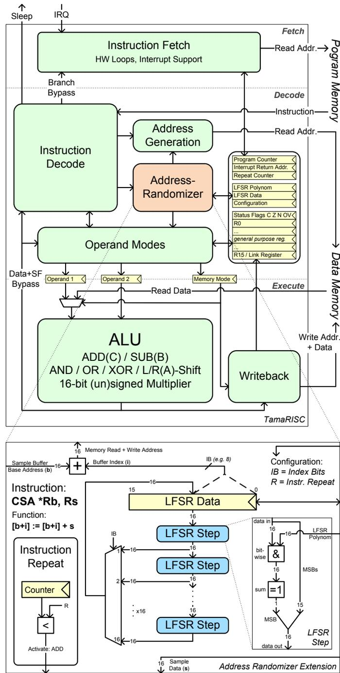
**Fig. 1.** TamaRISC sub-V<sub>T</sub> microprocessor architecture including address-randomizer extension for CS
