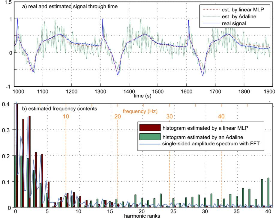
**Fig. 4.** Performances of a linear MLP with 3 hidden neurons, an Adaline and the FFT in identifying harmonics of an ECG.
