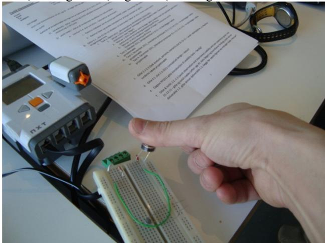
**Fig.11.** Testing and calibrating the light sensor
