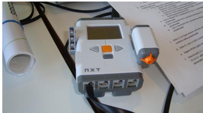
**Fig.5.** LegoMindstorms NXT as the platform for prototyping
