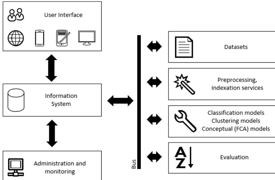
**Fig. 2** Architecture of text mining analytical system
