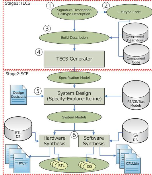
**Fig. 2.** Design flow using the proposed framework.
