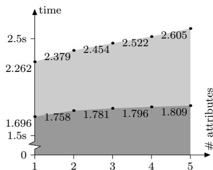
**Figure 3.** Credential issuance times (■: computations, ■: overhead; 1024 bits).
