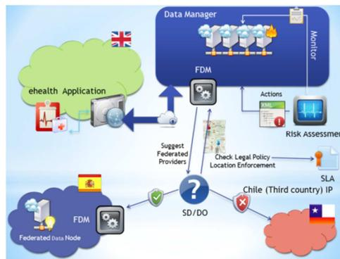
**Fig. 1.** OPTIMIS federation scenario: the home IP located in the UK may automatically select from a variety of providers located in the EU/EEA and compatible countries but not third countries even if the target IP is compliant but not adequately certified
