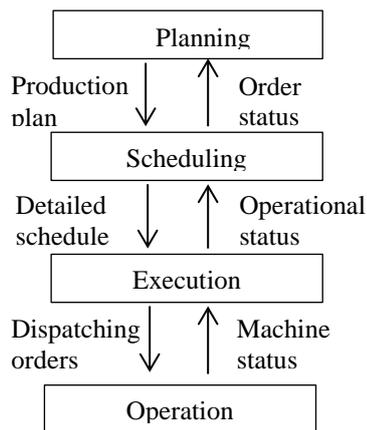
**Fig 1.** Hierarchical production control
