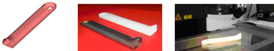
**Fig. 9.** Rapid prototyping from FE simulation result and control measurement on CMM
