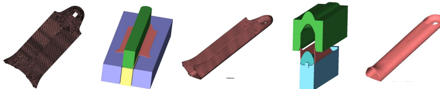
Fig. 6. Numerical models for FE analysis of virtual manufacturing
