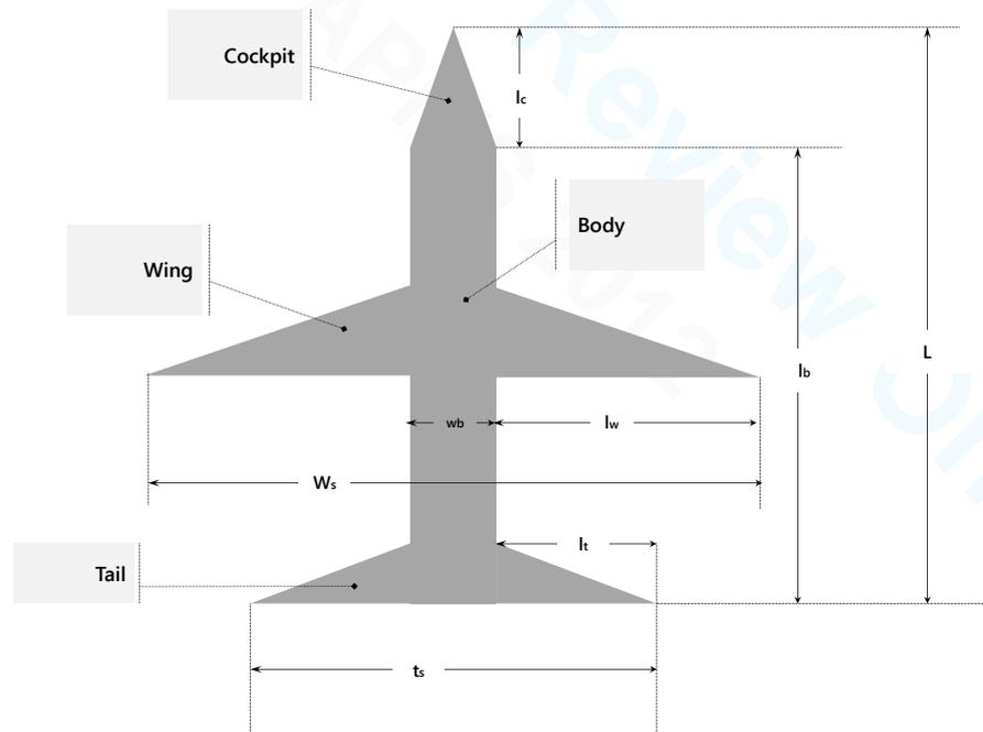
**Fig. 1.** A simplified airplane to be designed in the game (using LEGO bricks). "L": Length of Airplane, "lw": Length of Wing, "lb": Length of Body, "wb": Width of Body, "lc": Length of Cockpit, "Ws": Wing Span, "lt": Length of Tail, "ts": Tail Span
