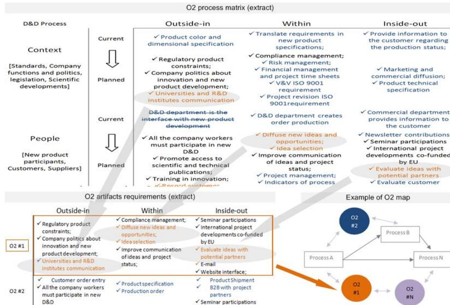
**Fig. 2.** The O<sub>2</sub> matrix (top), the O<sub>2</sub> artifacts (bottom-left), and an O<sub>2</sub> map (bottom-right) [27].
