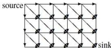
**Fig. 1.** Example of a  $3 \times 5$  grid DAG
