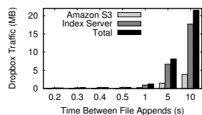
Fig. 6. Dropbox traffic as the time between 1 byte appends is varied (5400 RPM HDD).
