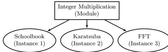
**Fig. 2.** Different Instances for the module *Integer Multiplication*.
