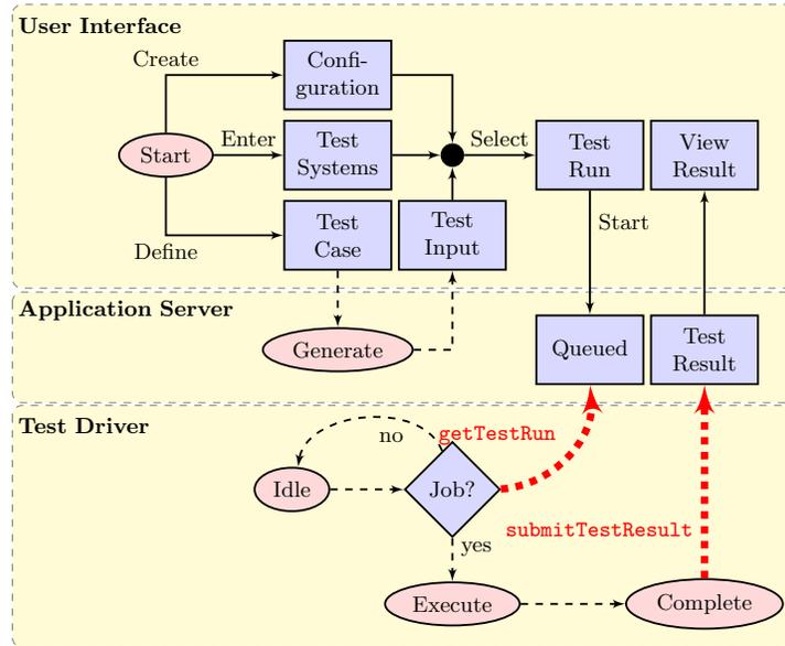
**Fig. 6.** Workflow when creating and executing a test run using *CaPTIF*. The figure shows the steps taken in the web interface (top), by the application server (middle), and by the test driver executing on the test systems (bottom). Dotted lines indicate automated events while solid lines are user actions.
