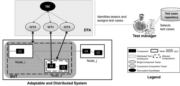
**Fig. 3.** Overview of a detailed Distributed Test Architecture.
