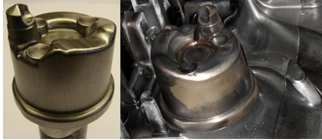
Fig. 13. - laser beam melted tool insert (left) and installed as a component in the die (right)
