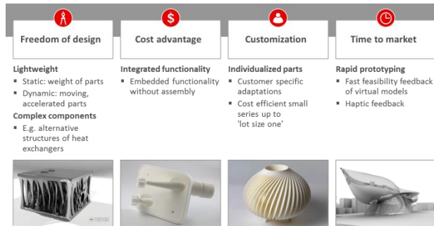
Fig. 3. - Key differentiation criteria for Laser Sintering
