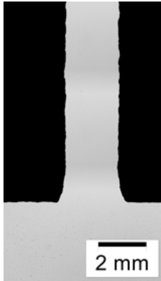
Fig. 3. Cross-section of a laser generated wall of INCONEL718
