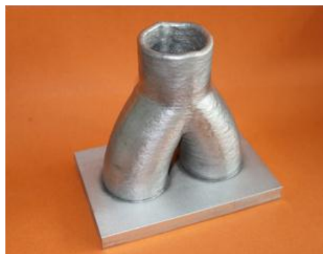
Inlet tube out of AlMg5
