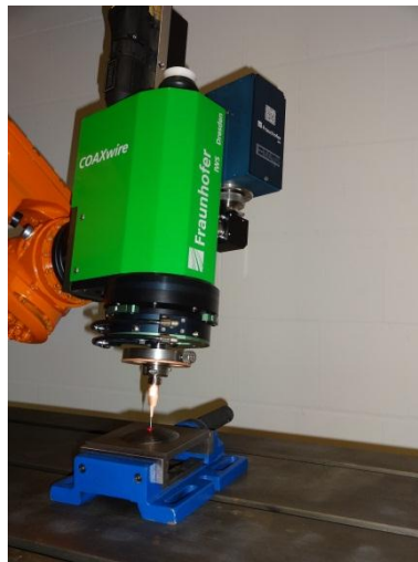
Fig. 1. Laser processing optic with coaxial wire supply
