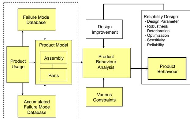
**Fig. 9.** - Model based engineering with disturbances [7]
