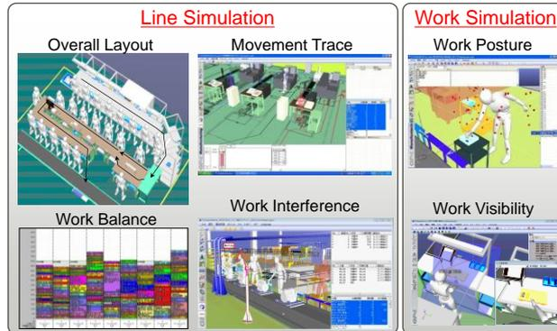
**Fig. 8.** - Digital Pre-Validation of Production Lines [6]
