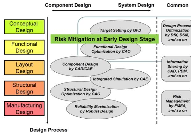
Fig. 6. - 1DCAE approach for large system design [5]
