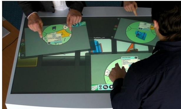
Fig. 3. - Multi-User Multitouch environment for design reviews.
