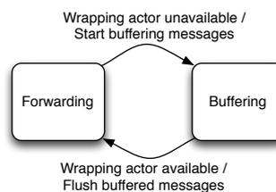
**Fig. 3.** State diagram for an undead reference
