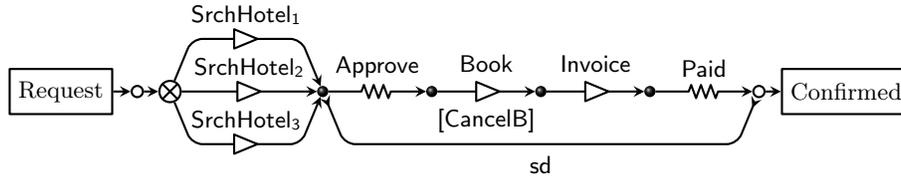
**Fig. 1.** Example of a Hotel Reservation workflow. Nodes (●) receive data from exactly one of their inputs, and replicate it to all of their outputs. The exclusive router (⊗) is a special node that forwards data to exactly one of its outputs. Transformer channels are represented using a triangle and filter channels using a zig-zag line.
