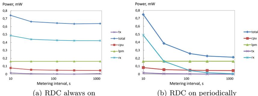
**Fig. 2.** Power consumption at a constrained device, both total and according to modes of operation including CPU active (cpu), low power mode (lpm), transmission (tx), and reception (rx): (a) RDC always on; (b) RDC on periodically. Note that a logarithmic scale is used for the metering interval shown on the x-axis.
