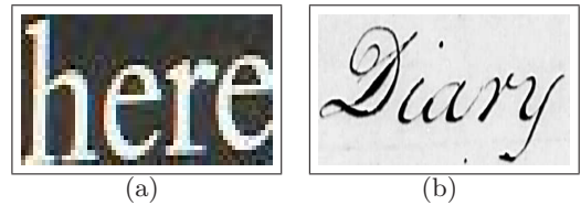
Fig. 2. (a) A scene text image from ICDAR 2013 dataset [22], and (b) part of a handwritten document image taken from H-DIBCO 2012 [11]. We note that stroke width within text is not always constant, and varies smoothly.
