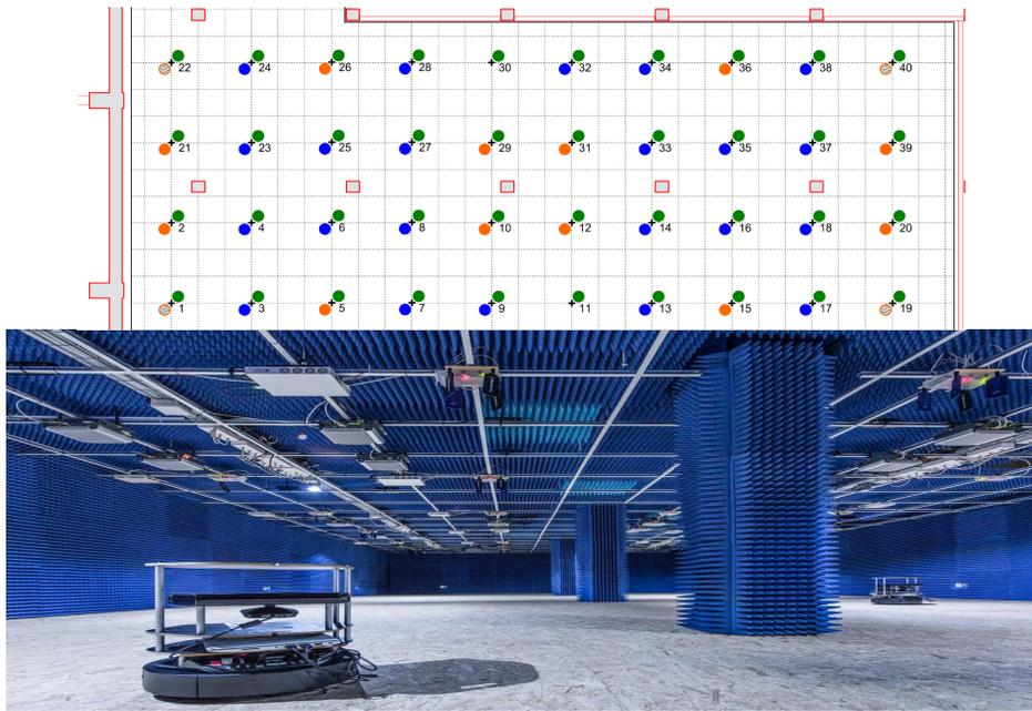
Fig. 4. CorteXlab platform and the nodes placement map.
