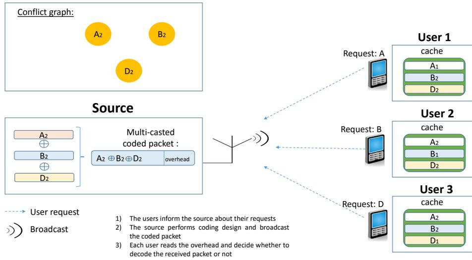
Fig. 2. Joint design of caching-aided coded multicasting in a 3-user SLN where each user is equipped with a storage capacity of 1.5 file and requests one file from a library with 4 binary files.
