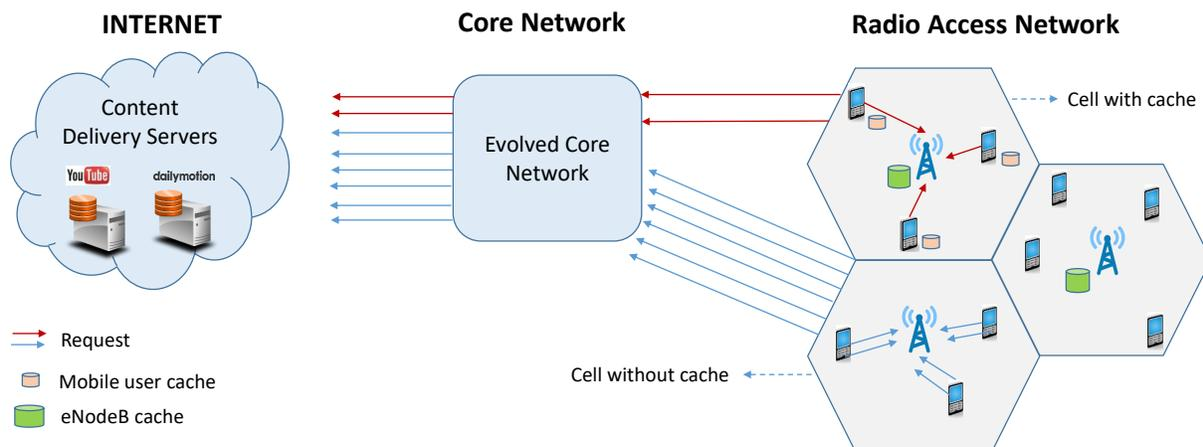
Fig. 1. Caching within the radio access network: impact on network load and traffic congestion.
