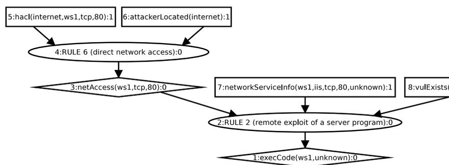
**Fig. 3.** Example of MulVAL attack tree [5]
