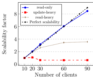
Fig. 3: Scalability of 10 RAMCloud servers in terms of throughput when varying the clients number. The “perfect” line refers to the expected throughput when increasing the number of clients. We take the baseline as the throughput achieved by 10 clients.
