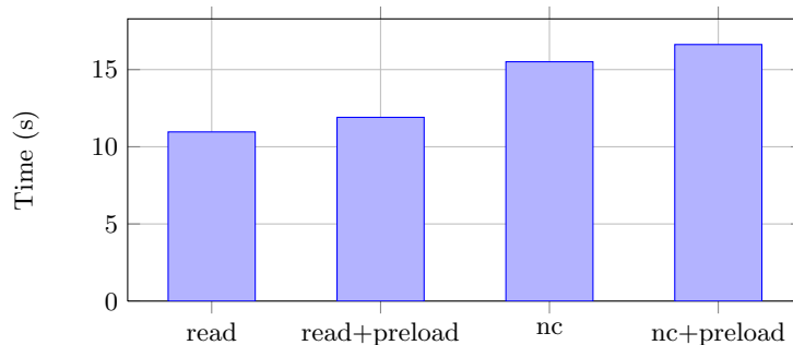
Fig. 2: Average time to run 20.000 times tests with library preload enabled/disabled
