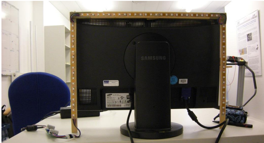
Fig. 4. LED-Frame mounted on the backside of the monitor
