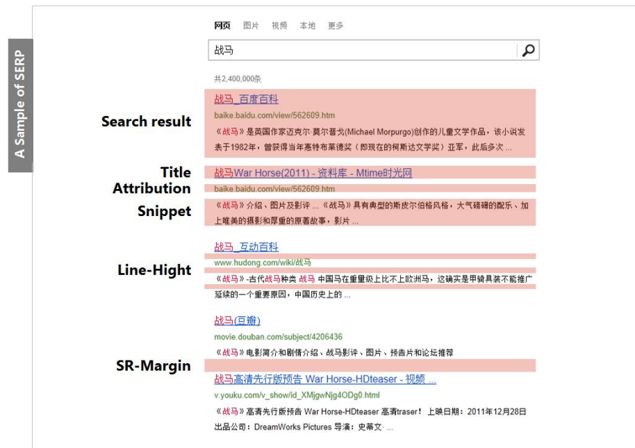
Fig. 1. An illustration of the terms of the line height, the SR-margin, and the title, attribution, and the snippet of search results
