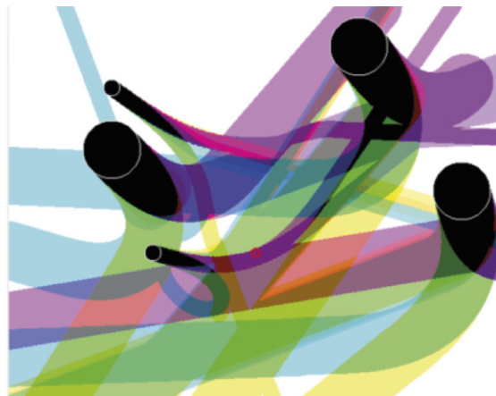
Figure 1: A self-driving vehicle among fixed and moving obstacles (left); 2D slice of the 5D state space of the self-driving vehicle, the black areas are the corresponding inevitable collision states that must be avoided (right).
