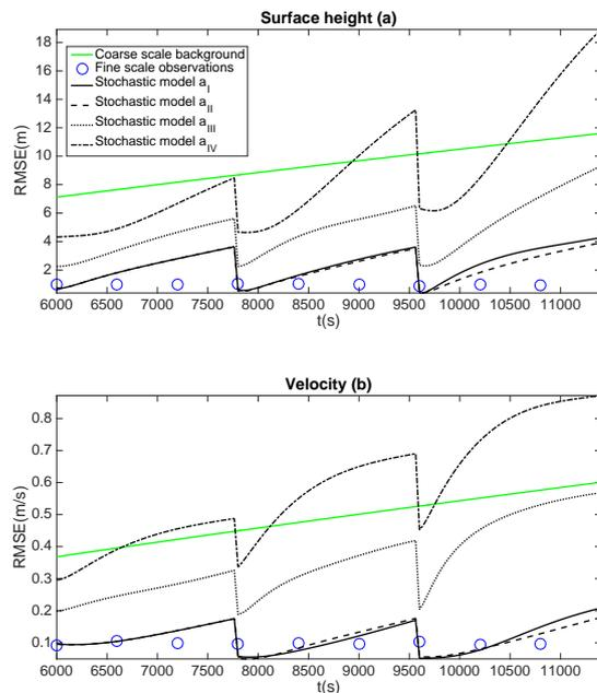
Fig. 4. RMSE comparison in terms of free surface height (a) and velocity (b) between various subgrid model configurations in table 1 of stochastic shallow water model (17). The meaning of different  $\alpha$  is shown in table 1.
