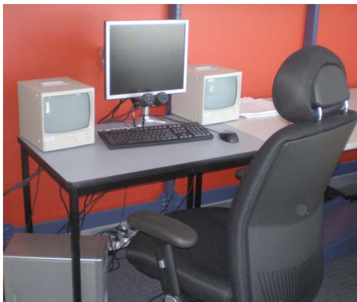
Fig. 7. Gaze tracking setup
