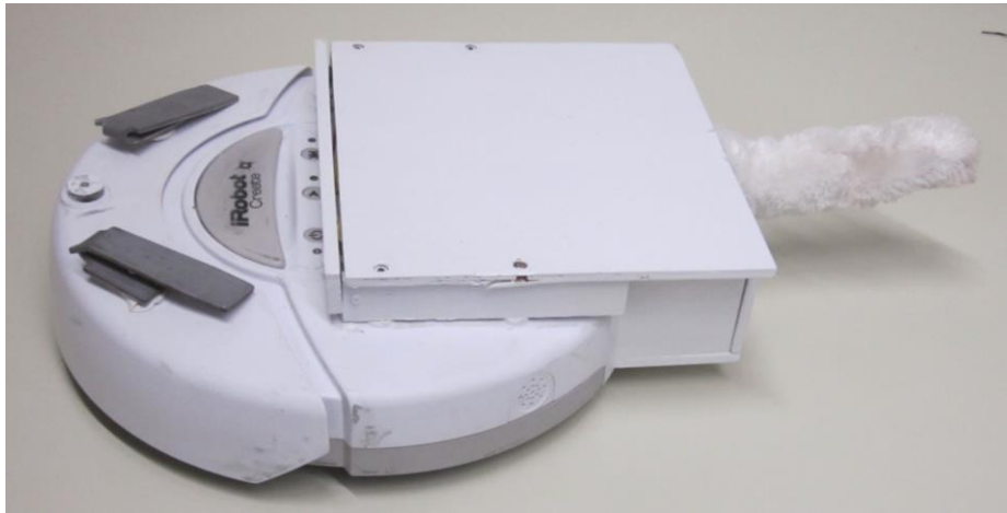
Fig. 2. An iRobot Create with our dog-tail attached.
