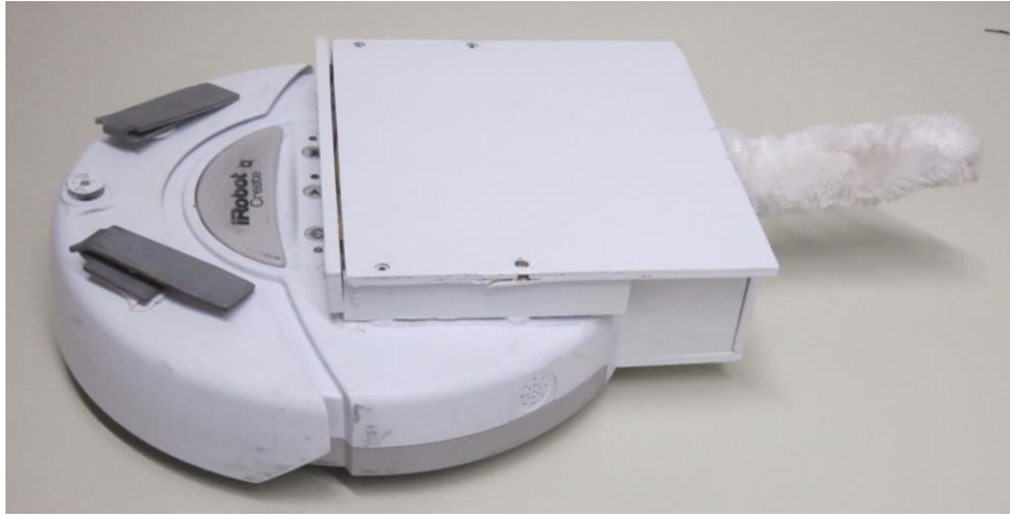
Fig. 2. An iRobot Create with our dog-tail attached.
