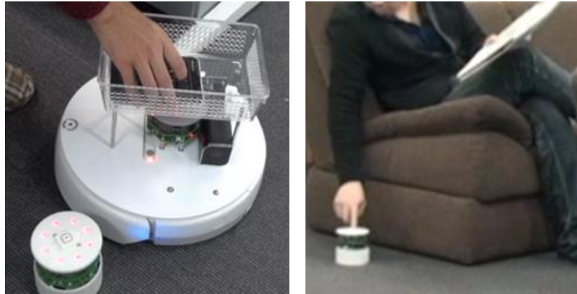
Fig. 6. Two Ways to Specify a Goal. The user can specify a goal of the robot by pressing a button on the remote control attached to the robot (left). The user can also specify a goal by pressing the button of the pebble (right).
