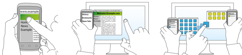
Fig. 2. (left) The mobile user interface allows for the display of a limited amount of information. (middle) Connecting the mobile and an external display extends the available screen space. (right) Items can be shared with others via drag-and-drop to another connected mobile device.
