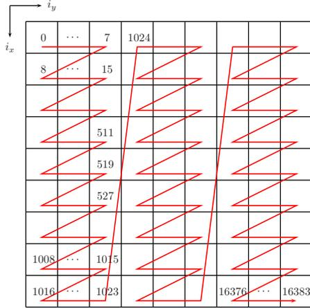
Figure 4. L4D layout of a 128 x 128 matrix, SIZE=8.
