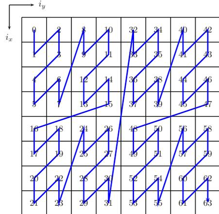
Figure 3. Morton layout of a 8 x 8 matrix.
