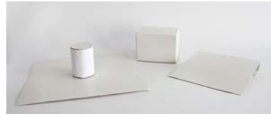
Fig. 2. Paper prototypes mimicking a knob, a gesture tracking device and a touch sensitive surface.
