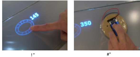
Fig. 7. The strip board allows for the investigation of other input devices such as (a) a static raised area on the board for entering flight headings or (b) a device with three LED's that can be placed anywhere on the board
