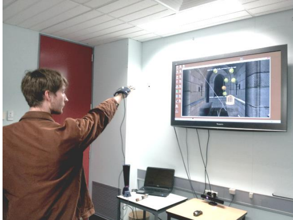
Fig. 1. Selecting a firefly in the select-drag-drop trial using the P5 Wired Glove
