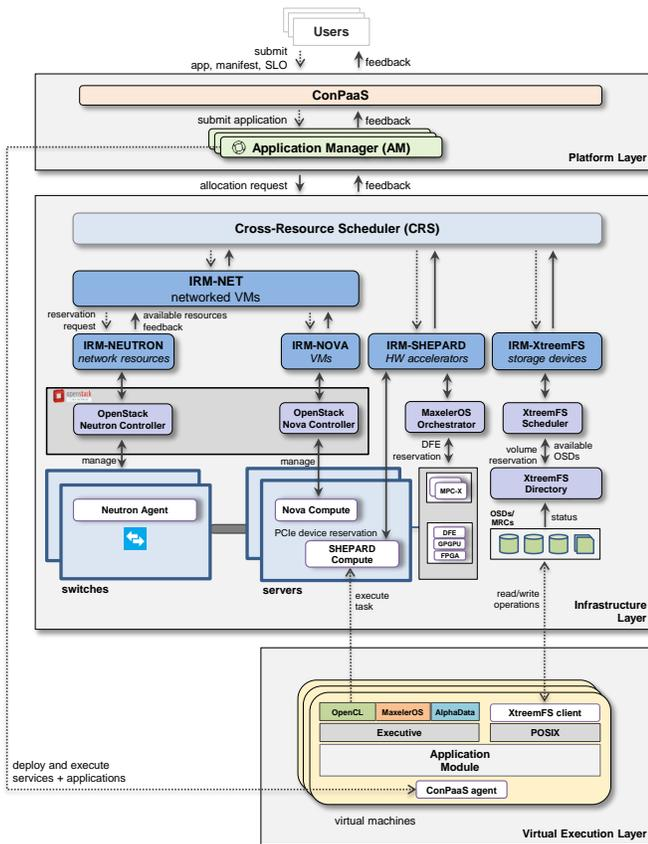
Figure 8: The HARNCESS architecture is composed of three layers: a platform layer that is responsible for managing applications, an infrastructure layer where cloud resources are managed, and a virtual execution layer where applications are deployed and executed.
