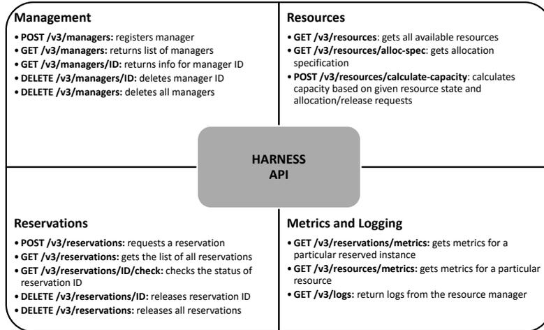
Figure 7: The HARNCESS API provides a REST-based interface for top-level resource managers to handle heterogeneous resources.
