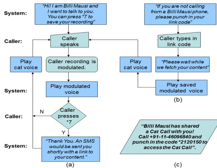
**Fig. 1.** Interaction tree of sharing voice site content, a) calling the general application and creating a recording b) calling the application to retrieve stored content, c) example SMS as received by our users.
