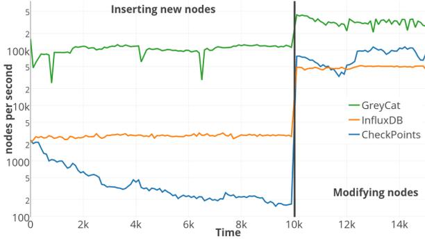
Fig. 3. Write throughput when creating and updating nodes
