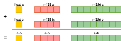
FIGURE 3: Summation example of single precision floating-point values using : (■) scalar standard C++ code, (■) SSE SIMD-vector of 4 values , (■) AVX SIMD-vector of 8 values.
