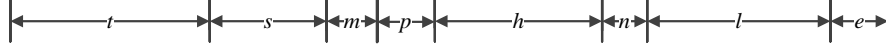
Fig 2. HTTP log structure, where t is the timestamp, s is source IP, m is method, h is hostname, p is protocol, n is port, l is path and e is web page's file type.
