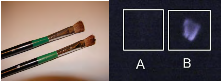
Fig. 6. Left: dry brush A (12mm) and wet brush B (10mm). Right: the infrared footprint of the two brushes. Notice the clear footprint image for the wet brush B caused by frustrated total internal reflection. Dry brush A does not generate a footprint image.
