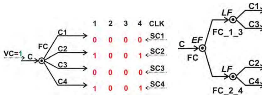
Fig. 22. Stall patterns at the branches of FC in the presence of bubbles.
